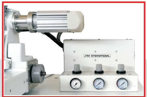
PRESSURE REGULATORS FOR FOOT AND PULLER - DIRECT DRIVE MOTOR
